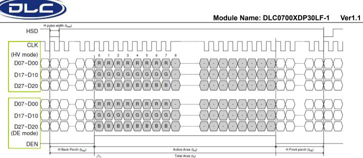
Figure: Horizontal input timing diagram
