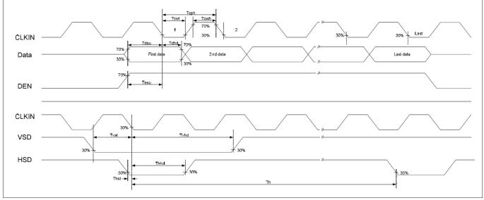
Figure: Input clock and data timing diagram
