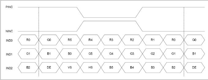
Figure: 6-bit LVDS input
