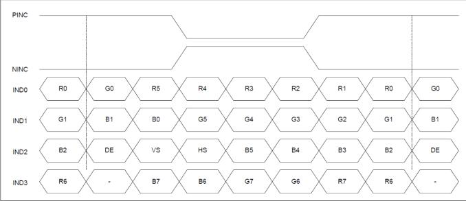
Figure: 8-bit LVDS Input
